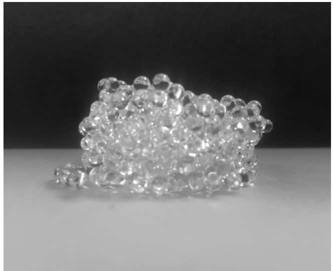
FIG. 1. Example of a cohesion-controlled granular material: a pile of glass beads d = 3 \text{ mm} with a PBS coating layer of thickness b = 2.2 \text{ }\mu\text{m}
