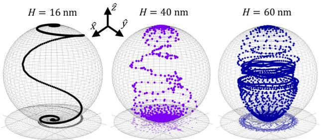
FIG. 3. Switching trajectories of magnetization of the storage layer represented on the unitary sphere. The  $z$  axis represents  $\langle m_z \rangle$  and the basal plane ( $x$  and  $y$  axes) represents  $\langle m_{x,y} \rangle$ . Results obtained for an applied voltage of  $-3$  V; pillar heights of 16, 40, and 60 nm, and constant base width of  $W = 20$  nm.
