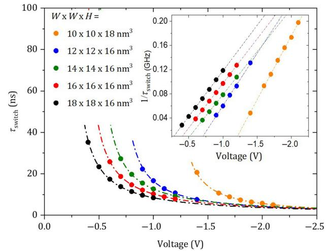
FIG. 8. Dependence of switching time on applied voltage for different studied aspect ratios (1.8, 1.3, 1.1, 1.0, and 0.9). Inset shows the dependency of inverse switching time on applied voltage.
