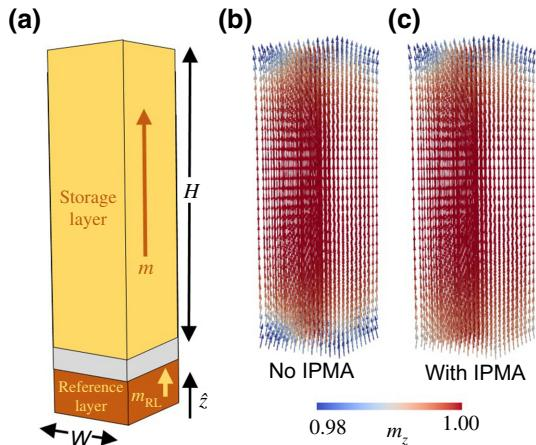
FIG. 1. (a) Three-dimensional (3D) scheme of the studied Fe-Co-B prism with height  $H$  and base width  $W$ . Storage layer is shown with a yellowish color, tunnel barrier with a gray color, and reference layer with a reddish color. 3D equilibrium initial state of 60-nm-thick Fe-Co-B layer (b) without IPMA and (c) with IPMA. Color bar indicates normalized magnitude of magnetization along the defined  $z$  direction (along the square-prism axis) in each computational cell.
