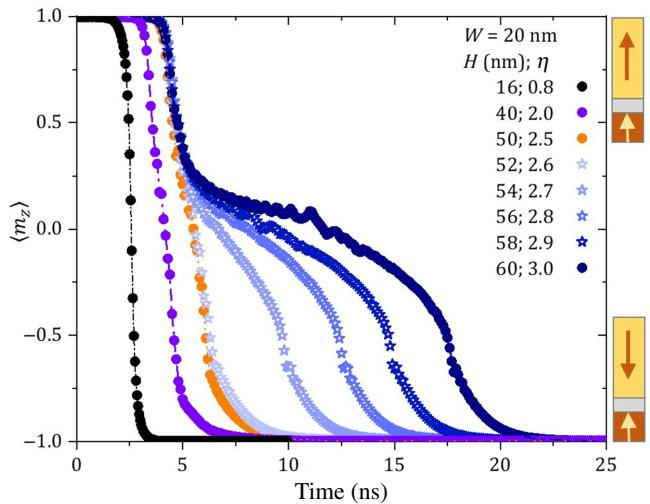
FIG. 2. Time traces of mean reduced magnetization  $\langle m_z \rangle$  for a storage layer with a constant base width of  $W = 20$  nm, variable height  $H$ , and aspect ratio  $\eta$ . Applied voltage is  $-3$  V.
