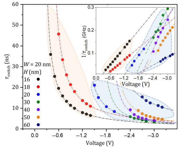
FIG. 5. Dependence of switching time on applied voltage for different heights of the storage layer and constant base width of  $W = 20$  nm. Coherent reversal is highlighted in light pinkish and noncoherent in light blue. Inset shows the dependency of the inverse switching time on applied voltage.
