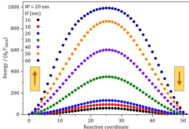
FIG. 6. Minimum-energy path between up and down states for different heights of the storage layer with constant base width of 20 nm.
