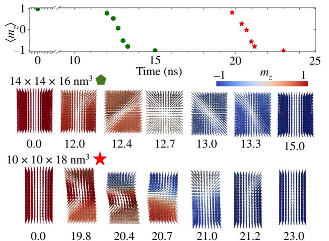
FIG. 7. Snapshots of magnetization at different time steps in ns (in bold, time to reverse 10%, 50%, and 90% magnetization). Bottom line, pillar with  $W = 14$  nm and  $H = 16$  nm at an applied voltage of  $-1$  V. Middle line, pillar with  $W = 10$  nm and  $H = 18$  nm at an applied voltage of  $-1.4$  V. Color bar is linked to  $m_z$  and time steps selected are displayed on the time trace of average magnetization plot at the top with associated symbols.
