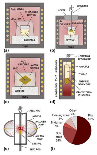
**Figure 3:** Schematic representation of growth methods for KNN-based single crystals: (a) seed-less solution (flux) growth, (b) TSSG, (c) SSCG (with seed), (d) Bridgman–Stockbarger method, and (e) floating zone method (with mirror furnace). (f) Percentages of publications on KNN-based crystals for individual growth method.
