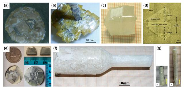
**Figure 4:** Examples of KNN-based single crystals, grown by different methods: (a) seed-less self-flux method [45], (b) self-flux growth using Pt spatula as nucleation site [46], (c) TSSG [47, 48], (d) solid-state crystal growth with KTaO<sub>3</sub> seed [49], (e) seed-free solid-state crystal growth [50], (f) modified Bridgman method [51], and (g) floating zone method [52]. Note the different scales on the pictures.
