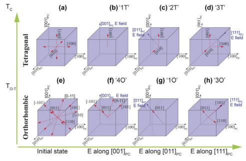
Figure 8: Domain configurations of tetragonal and orthorhombic phases under various conditions: (a, e) initial state and E-field applied along (b, f) [001]<sub>PC</sub>, (c, g) [011]<sub>PC</sub>, and (d, h) [111]<sub>PC</sub> direction.
