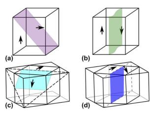
**Figure 9:** Schematics for exemplary domain walls appearing in perovskite ferroelectrics with tetragonal structure: (a) 90° domain wall on (101) plane, (b) 180° domain wall and orthorhombic structure (c) 60° domain wall on (111)<sub>0</sub> plane, and (d) 90° domain wall on (110)<sub>0</sub> plane. Redrawn from Refs. 121 and 123.
