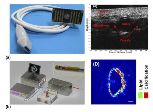
Figure 11: Examples of transducers and corresponding images: (a) 30 MHz KNbO3-based transducer used to perform in vivo imaging of human forearm skin (© 2019 IEEE. Reprinted, with permission, from Ref. 157.), (b) the photoacoustic probe for intravascular imaging using KNN single crystals and a reconstructed image of a calcified atherosclerotic human artery (scale bar is 1 mm) (reprinted from Ref. 158).
