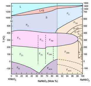
**Figure 2:** Phase diagram of the KNN system [32, 33]. Symbols and subscripts: L, liquid; S, solid; P, paraelectric; C, cubic, T, tetragonal; O, orthorhombic; MON, monoclinic; TM, pseudotetragonal; and R, rhombohedral (reprinted with permission from Wiley).
