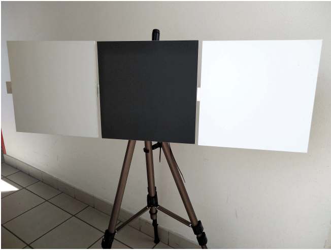
Fig. 5. The reference targets grey (50%), black (5%) and white (90%) Zenith Polymer from Pro-Lite Technology.
