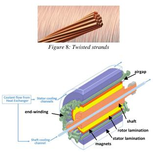
Figure 9: High specific power electric motor section
