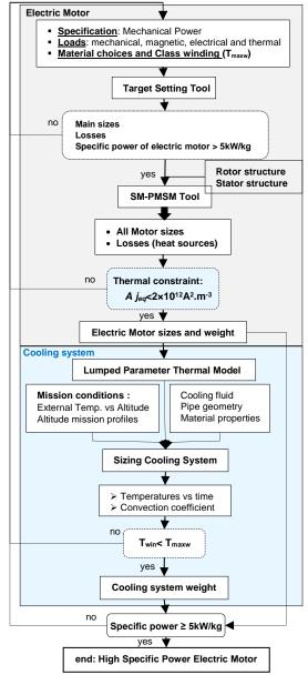
Figure 3: Interaction between Electro-thermal models for sizing high specific electric motor with its cooling system
