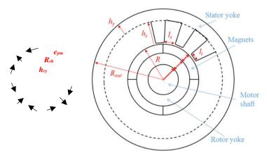
Figure 2: Sizes given by SM-PMSM Tool
