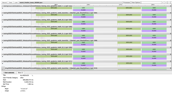
Fig. 3. Horovod timeline: An example of the visual representation of the events generated by the ResNet-50 benchmark
