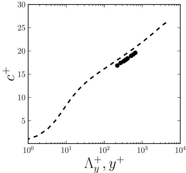
FIG. 4. Neutral log-layer modes for  $Re_\tau = 5000$  and  $\lambda_z^+$  ranging from 1420 to 3500 ( $\bullet$ ): the phase speed in the streamwise direction  $c^+$  is shown as a function of the vertical length scale  $\Lambda_y^+$ . The dashed line represents the mean streamwise velocity as a function of the wall-normal direction  $y^+$ .
