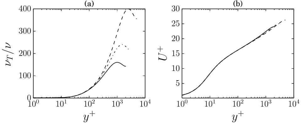
FIG. 1. (a) Cess eddy viscosity and (b) streamwise turbulent velocity profile plotted as a function of the distance normal to the wall scaled in wall units for  $Re_\tau = 2000$  (—),  $3000$  (---), and  $5000$  (-·-·-·).
