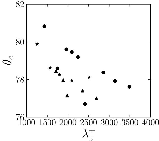
FIG. 14. Neutral log-layer mode: distribution of the maximum streak lift angle as a function of the spanwise wavelength scaled in inner units for  $Re_\tau = 2000, 3000,$  and  $5000$  ( $\blacktriangle$ ,  $\star$ , and  $\bullet$ , respectively).
