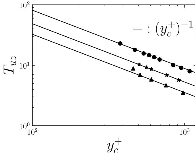
FIG. 9. Neutral log-layer modes: distribution of the production term  $T_{uz}$  associated with the work of the Reynolds stress against the spanwise shear as a function of the distance from the wall  $y_c^+$  for  $Re_\tau = 2000, 3000,$  and  $5000$  ( $\blacktriangle$ ,  $\star$ , and  $\bullet$ , respectively).
