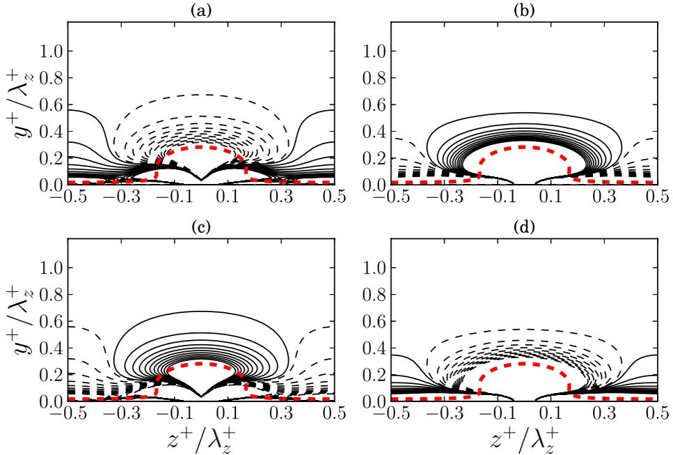
FIG. 12. The normal vorticity component associated with the critical log-layer mode for  $Re_\tau = 5000$  and  $\lambda_z^+ = 2244$  at (a)  $\alpha x = 0$ , (b)  $\alpha x = \pi/2$ , (c)  $\alpha x = \pi$ , and (d)  $\alpha x = 3\pi/2$ . Solid (dashed) lines represent positive (negative) contours. The critical layer position is shown in red thick dashed lines.
