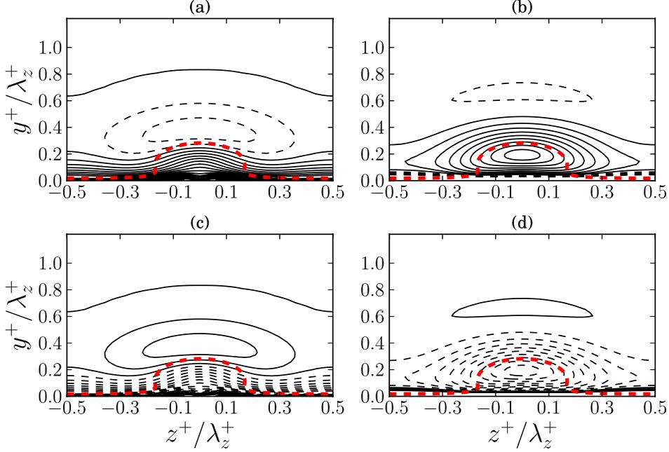
FIG. 10. The streamwise vorticity component associated with the neutral log-layer mode for  $Re_\tau = 5000$  and  $\lambda_z^+ = 2244$  at (a)  $\alpha x = 0$ , (b)  $\alpha x = \pi/2$ , (c)  $\alpha x = \pi$ , and (d)  $\alpha x = 3\pi/2$ . Solid (dashed) lines represent positive (negative) contours. The critical layer position is shown in red thick dashed lines.
