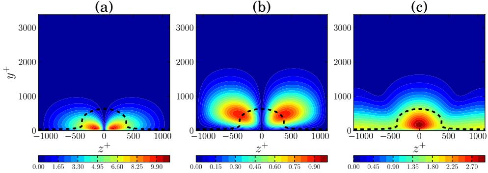
FIG. 5. Cross-stream ( $y^+ - z^+$  plane) view of the eigenfunctions associated with the neutral log-layer mode for  $Re_\tau = 5000$ ,  $\lambda_z^+ = 2244$ , and  $\lambda_x^+ = 6000$ . (a)  $|u|$ , (b)  $|v|$ , and (c)  $|w|$ . The position of the critical layer is also shown in dashed lines.
