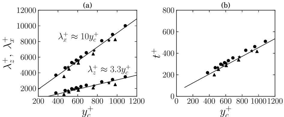
FIG. 6. Neutral log-layer modes: (a) spanwise and streamwise wavelengths and (b) convective time scale  $t^+ = \lambda_x^+/c^+$  reported as a function of the distance from the wall  $y_c^+$  for flow cases  $Re_\tau = 2000, 3000$ , and  $5000$  (▲, ★, and ●, respectively).
