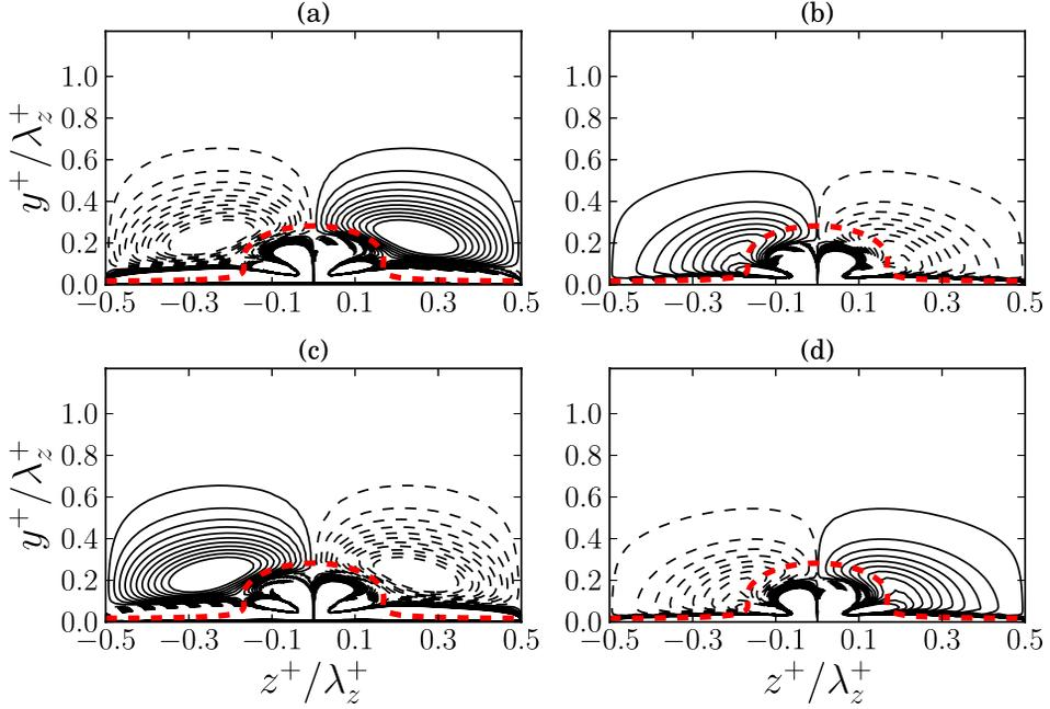
FIG. 11. The tangential vorticity component associated with the neutral log-layer mode for  $Re_\tau = 5000$  and  $\lambda_z^+ = 2244$  at (a)  $\alpha x = 0$ , (b)  $\alpha x = \pi/2$ , (c)  $\alpha x = \pi$ , and (d)  $\alpha x = 3\pi/2$ . Solid (dashed) lines represent positive (negative) contours. The critical layer position is shown in red thick dashed lines.
