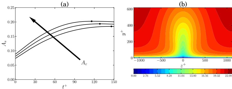
FIG. 2. Base flow simulations at  $Re_\tau = 5000$  and  $\lambda_z^+ = 2244$ . (a) Streak amplitudes vs time scaled in wall units for three initial amplitudes of optimal streamwise vortices  $A_v = 0.05, 0.055, \text{ and } 0.06$ . The maximum amplitude,  $(A_s)_{max}$ , is denoted by  $\bullet$ . (b) Streamwise velocity contours in wall units of the nonlinear saturated low-speed streak for the time indicated by  $\bullet$  in (a) and  $A_v = 0.05$ .
