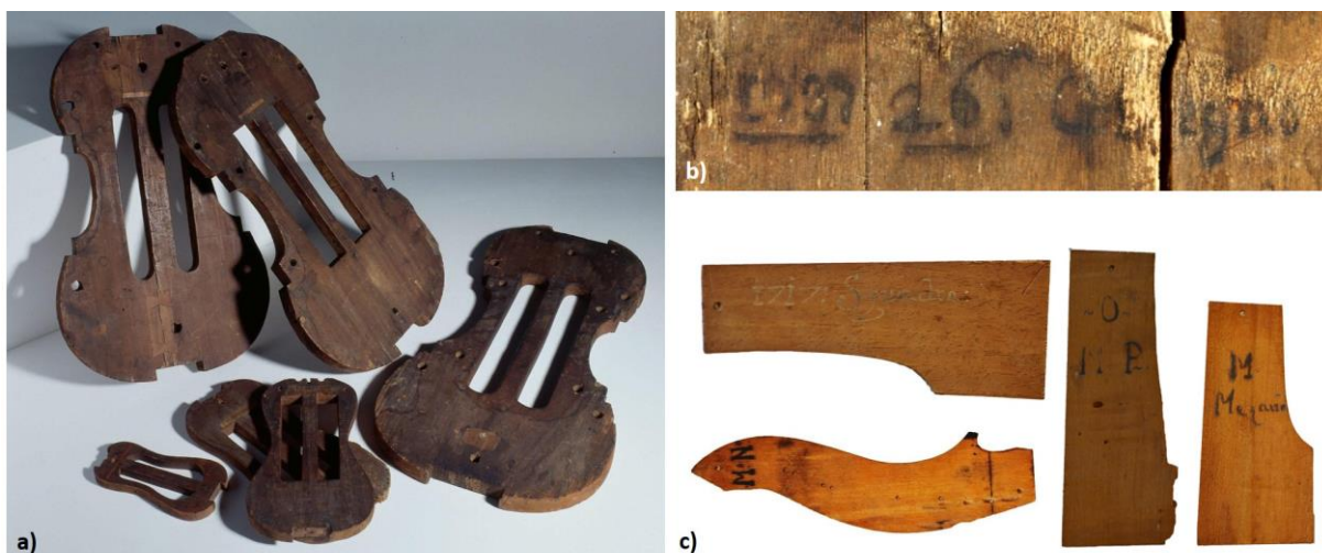
FIGURE 1. Visible pictures of (a) the six inner wooden forms, (b) a detail of an inscription on the form E.901.1, and (c) four of the eight smaller items with inscriptions. Collection Musée de la musique, Paris, France. Photos (a) C. Giordan, (b, c) Claude Germain © Cité de la musique - Philharmonie de Paris.
