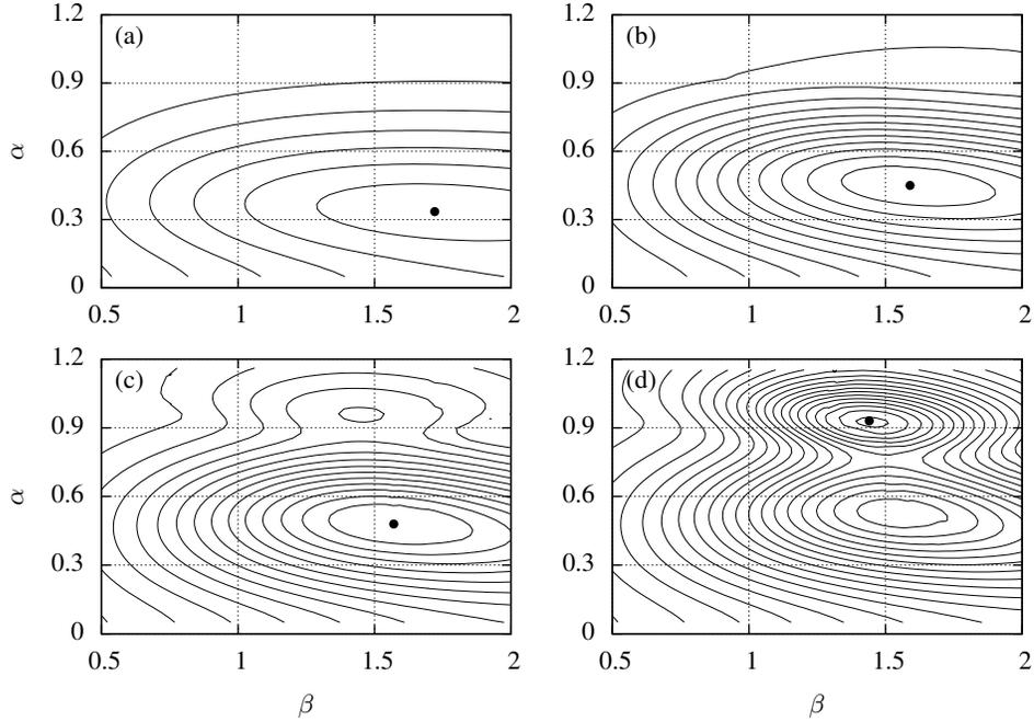
FIGURE 6. Gain  $G$  in the  $\alpha - \beta$  plane for  $Re = 400$  and  $T = 20$ ; (a)  $\epsilon \rightarrow 0$  with contour values from 20 to 120, (b)  $\epsilon = 0.0145$  with contour values from 20 to 240, (c)  $\epsilon = 0.0153$  with contour values from 20 to 300, (d)  $\epsilon = 0.01603$  with contour values from 20 to 380. The interval among adjacent isolines is  $\Delta G=20$  in frames. The maximum value of  $G$  for each  $\epsilon$  is denoted by a filled circle.
