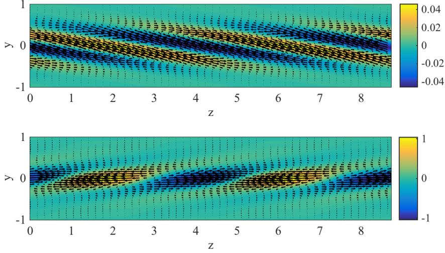
FIGURE 5. Vectors and contours, in the  $(y, z)$  plane, of the optimal oblique wave at  $t = 0$  (top) and at the target time  $T = 20$  (bottom), shown over two spanwise periods. The shaded contours represent the positive and negative streamwise velocity component, whereas the vectors represent wall-normal and spanwise components. Same parameters as in figure 3.
