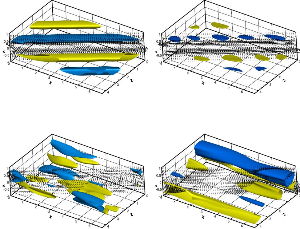
FIGURE 13. Isosurfaces of the streamwise perturbation to the base flow (yellow and blue for  $u = \pm 0.2$ , respectively), extracted from a DNS initialized with the optimal solution at  $t = 15$  for  $\epsilon = 0.0151$ . The snapshots are extracted at  $t = 25, 30, 45, 75$ .
