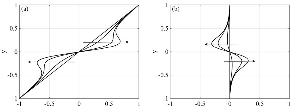
FIGURE 3. Components of the mean flow  $U + \epsilon^2 u_{00}$  (a) and  $\epsilon^2 w_{00}$  (b) at  $t = 0, 10, 15, 20$  for the case  $Re = 400$ ,  $\epsilon = 0.0153$ ,  $\alpha_{opt} = 0.93$  and  $\beta_{opt} = 1.44$ . The arrows display increasing values of  $t$ .
