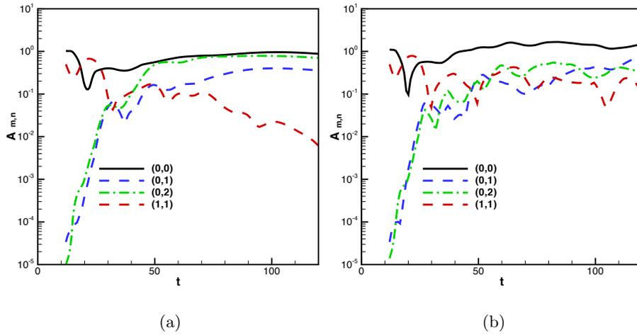
FIGURE 11. Variation in time of the amplitude of the different modes extracted by Fourier transform of the velocity snapshots obtained by DNS initialized with the weakly nonlinear solutions at  $t = 15$ ,  $\epsilon = 0.0151$  (a) and  $\epsilon = 0.0152$  (b). The legend indicates the streamwise and spanwise wavenumbers, as multiples of the  $\alpha$  and  $\beta$  values chosen for the optimisation.
