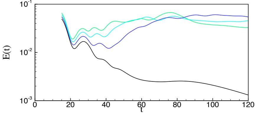
FIGURE 10. Disturbance energy  $E$  versus time measured by a DNS initialized with the weakly nonlinear optimal states at  $t = 15$ ,  $\epsilon = 0.0151, 0.0152, 0.0153, 0.0154$  (increasing from bottom to top).
