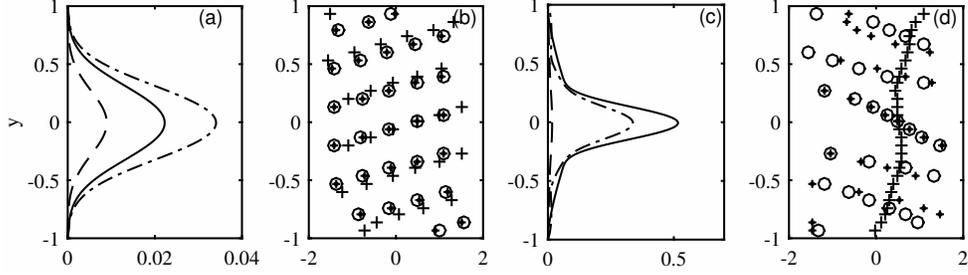
FIGURE 4. Modulus of velocity components and phase of the optimal oblique wave at  $t = 0$  (a,b) and its output at the target time  $T = 20$  (c,d). The  $u_{11}$ ,  $v_{11}$  and  $w_{11}$  components of the velocity are presented in (a,c) as solid, dashed and dash-dotted lines, respectively. The phase, in radians, of the  $u_{11}$ ,  $v_{11}$  and  $w_{11}$  components are shown in (b,d) as  $\circ$ ,  $+$  and  $*$ , respectively, and the parameters are those of figure 3.
