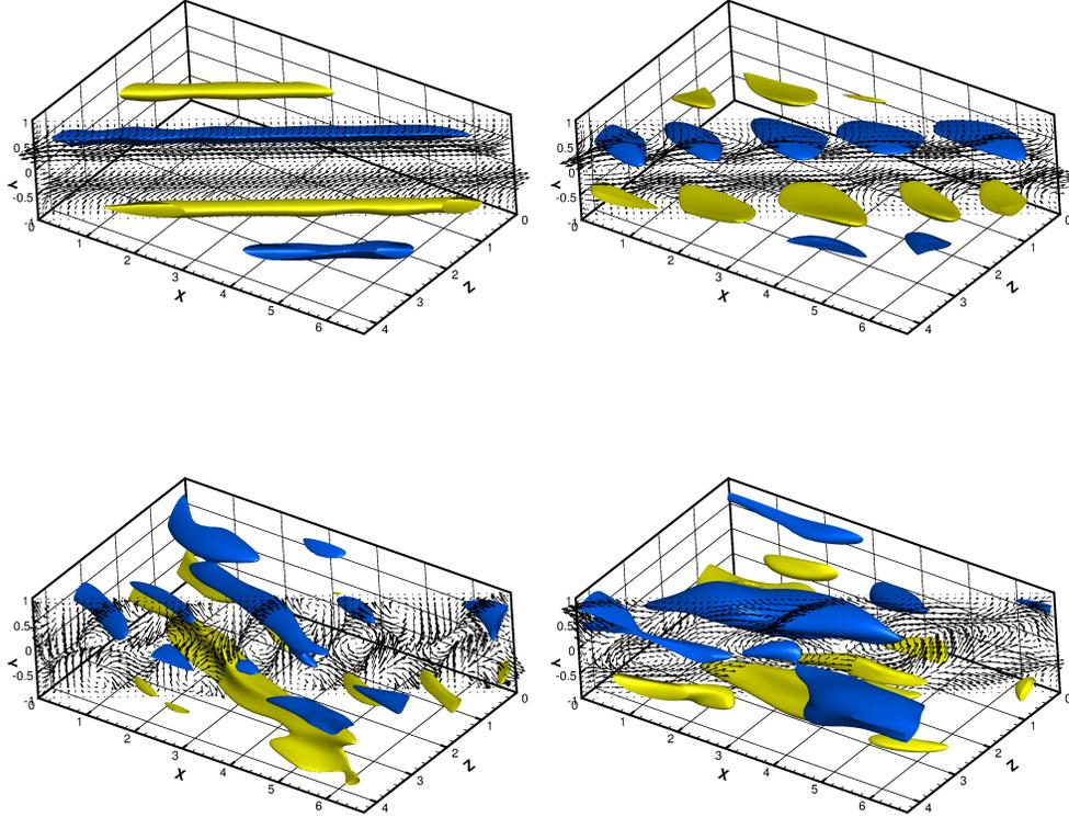
FIGURE 12. Isosurfaces of the streamwise perturbation to the base flow (yellow and blue for  $u = \pm 0.3$ , respectively), extracted from a DNS initialized with the optimal solution at  $t = 15$  for  $\epsilon = 0.0152$ . The snapshots are extracted at  $t = 25, 30, 35, 45$ .
