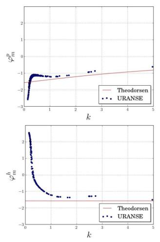
**Figure 11** Phase of the lift curve slope as a function of the reduced frequency for heave motion (left), and pitch motion (right)
