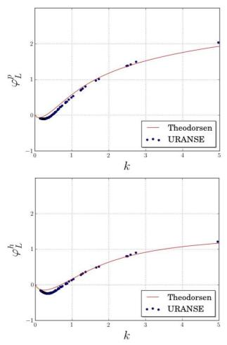
Figure 9 Phase of the lift curve slope as a function of the reduced frequency (pitch left, heave right)
