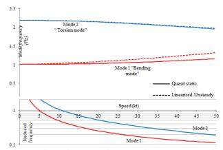
*Figure 12* Evolution of the natural frequencies of the keel as a function of speed (top), corresponding reduced frequencies
