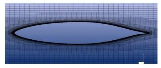
*Figure 4 Close view of the profile mesh*
