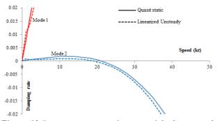
*Figure 13* Damping rate as a function of the boat speed, comparison between quasi-static and linearized unsteady hydrodynamic, (flutter speed is very close to 20 knots)
