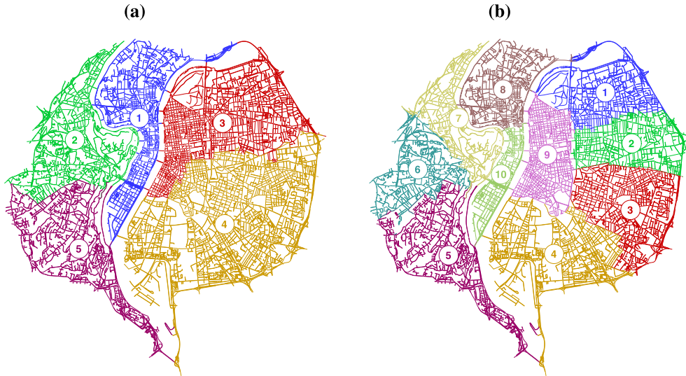
Fig. 4. (a) Road network of Lyon partitioned in 5 reservoirs, and (b) 10 reservoirs.
