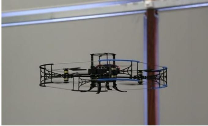
Fig. 2: The experimental Octorotor UAV
