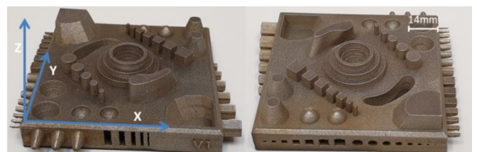
Fig. 4. Printed artefact (Z axis represents the building direction) [6]
