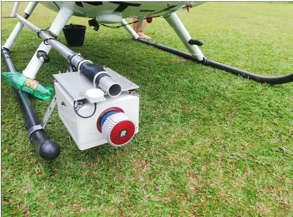
**Figure 4:** VUX-1 integrated into the Bell 500M helicopter.
