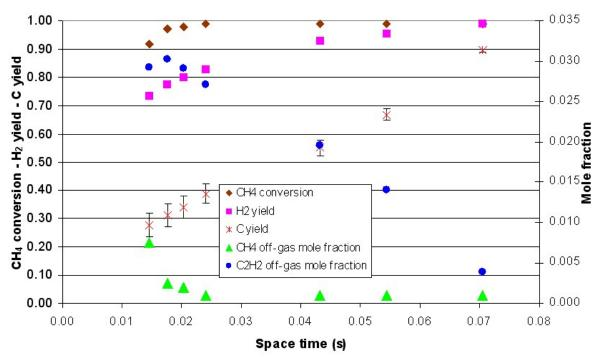
Fig. 5:  $CH_4$  conversion,  $H_2$  yield, C yield,  $CH_4$  and  $C_2H_2$  off-gas mole fractions versus space time (10 %  $CH_4$  in Ar)
