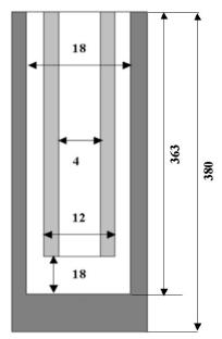
Fig. 2: Scheme of the tubular design (dimensions in mm, not scaled)
