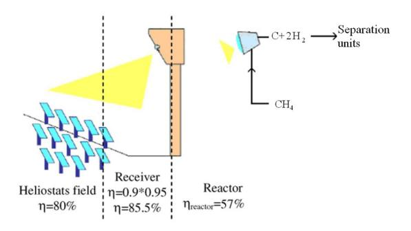
Fig. 6: Energy efficiencies related to the solar concentrating system, the receiver, and the reactor
