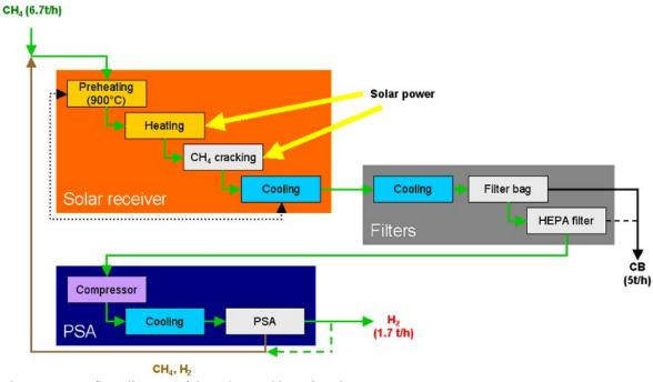
Fig. 7: Process flow diagram of the solar cracking of methane
