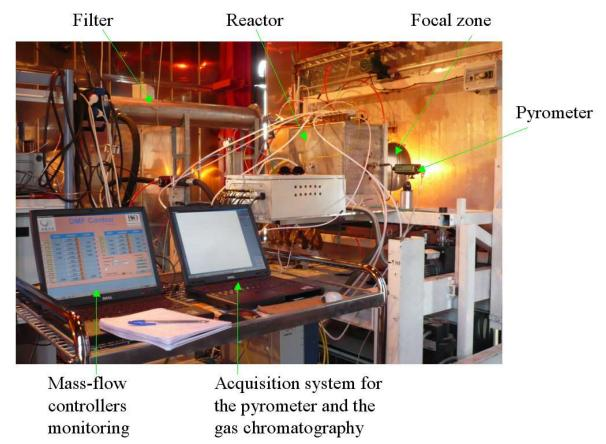
Fig 3: Photograph of the experimental set-up including the solar reactor
