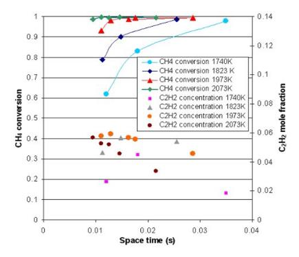
Fig. 4:  $CH_4$  conversion and  $C_2H_2$  off-gas mole fraction versus space time for various temperatures (20 %  $CH_4$  in Ar)
