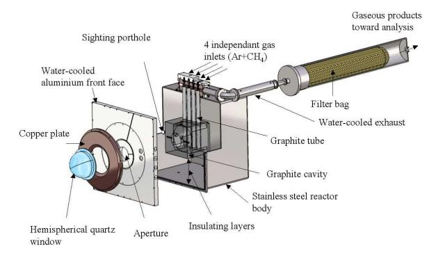
Fig. 1: Scheme of the 10 kW solar reactor and filter
