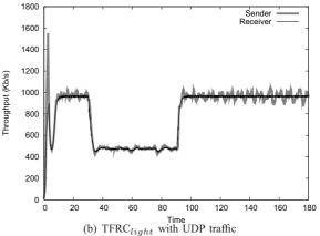
Fig. 9. TFRC and TFRC  $_{light}$  with a network bandwidth of 1Mbit/s, an RTT=100ms and introduction of an UDP flow at t=[30s,90s]
