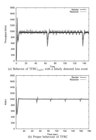
Fig. 5. Comparison of  $\mathrm{TFRC}_{light}$  with a false detection and a traditional TFRC implementation in a network with a bandwidth of 1Mbit/s, and an  $\mathrm{RTT} = 100ms$
