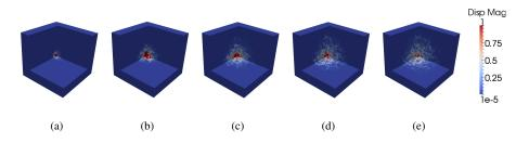
Figure 12: Normalized amplitude of the displacement field in a heterogeneous infinite medium at times: (a) t = 0.094 s; (b) t = 0.188 s; (c) t = 0.282 s; (d) t = 0.329 s; (e) t = 0.470 s.
