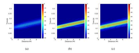
Figure 14: Displacement magnitude in an infinite homogeneous medium over different frequency ranges: (a) 0-50 Hz; (b) 50-100 Hz; (c) 100-150 Hz. The color scale is the amplitude of the displacement field, limited to values above -80 dB.
