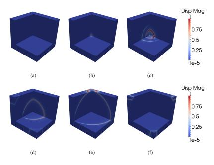
Figure 3: Normalized displacement fields in an infinite elastic isotropic homogeneous model at times: (a) t = 0.000 s; (b) t = 0.141 s; (c) t = 0.282 s; (d) t = 0.423 s; (e) t = 0.564 s; (f) t = 0.705 s.
