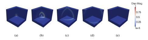
Figure 11: Normalized amplitude of the displacement field in a homogeneous infinite medium at times: (a) t = 0.094 s; (b) t = 0.188 s; (c) t = 0.282 s; (d) t = 0.329 s; (e) t = 0.470 s.
