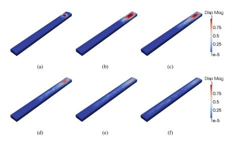
Figure 7: Normalized displacement fields in the ballasted railway track at times: (a) t = 0.135 s; (b) t = 0.225 s; (c) t = 0.315 s; (d) t = 0.405 s; (e) t = 0.495 s; (f) t = 0.585 s.
