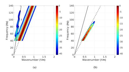
Figure 13: Dispersion curves for infinite homogeneous (figure (a)) and heterogeneous media (figure (b)). The color scale is the amplitude of  $H_{pq}$  evaluated in Eq. (5), limited to values above -40 dB. The dotted black line is the analytical solution for the homogenized pressure waves dispersion relation. The dashed black line is the analytical solution for the homogenized shear wave.
