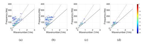
Figure 9: Dispersion curves for individual maps: for two different lines in the same realization of the ballast layer (no average, figures (a) and (b)), and for two different realizations of the ballast layer (averaged over the 6 lines for that realization, figures (c) and (d)). Dispersion relations for the homogenized ballast shear wave (black solid line) and soil shear wave (black dashed line) are also indicated. The color scale is limited at -40dB.
