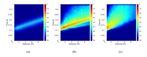
Figure 15: Displacement magnitude in an infinite heterogeneous medium over different frequency ranges: (a) 0-50 Hz; (b) 50-100 Hz; (c) 100-150 Hz. The color scale is the amplitude of the displacement field, limited to values above -80 dB.
