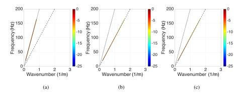
Figure 4: Dispersion curves for an infinite homogeneous media along axes x (figure a), y (figure b) and z (figure c). The color scale is the amplitude of  $H_{pq}$  evaluated in Eq. (5), limited to values above -25 dB. The dotted black line is the analytical solution for the pressure waves dispersion relation. The dashed black line is the analytical solution for the shear wave.
