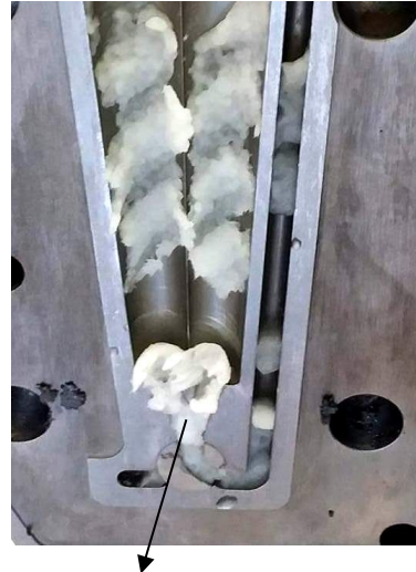
The fibers stack at the extremity of the screw, forming a plug that prevents the material from recirculating through the channel
