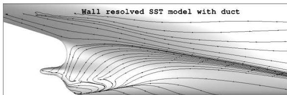
Fig.13: Wall streamlines with SST closure
