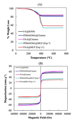
**Figure 8** – (A) TGA and (B) SQUID analyses of the commercial fatty acid-modified IO nanoparticles (FA@IONPs), the PDMAEMA@Clusters, the PAA@Clusters, and the magnetic fraction ( $\omega_{mag}$ ) of the PDMAEMA@MLPs and PAA@MLPs samples (Exp 7, Table 1 and Exp 11, Table 2).
