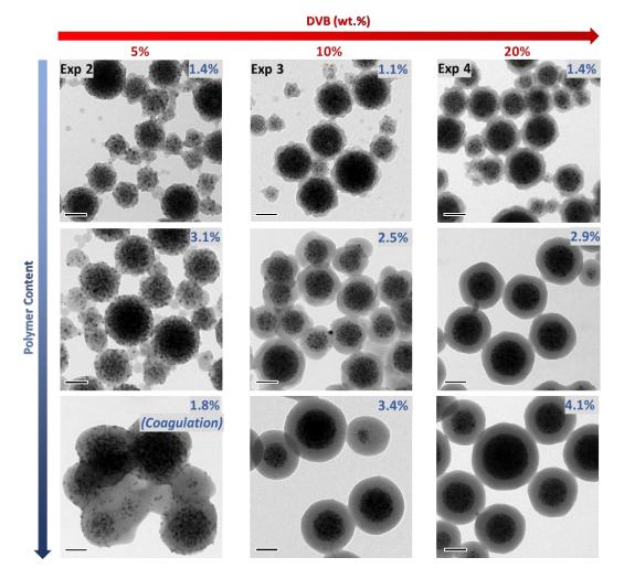
**Figure 4** – TEM micrographs of PDMAEMA@MLPs ( $PC_{theo} = 10 \%$ ) synthesized in the presence of increasing amounts of DVB (based on overall monomer mass): 5 wt%, 10 wt% and 20 wt% (Exp 2, 3 and 4, respectively, Table 1). The images from top to bottom correspond to samples taken at different reaction times and therefore, to increasing polymer contents. Scale bar: 100 nm.
