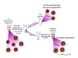
Figure 2 – Scheme of magnetic separation of IO/polymer composite latex particles.
