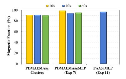
**Figure 9** – Magnetic fraction ( $\omega_{mag}$ ) obtained at different times of magnetic separation for the PDMAEMA@Clusters, and the PDMAEMA@MLPs (Exp 7) and PAA@MLPs (Exp 11) samples obtained by seeded emulsion polymerization of styrene (Tables 1 and 2).
