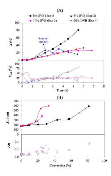
**Figure 3** – Effect of DVB content on (A) the instantaneous ( $X_{inst}$ , empty symbols) and global conversions (X, filled symbols) with time and (B) the particle size ( $Z_{av}$ , filled symbols) and size dispersity (PdI, empty symbols) with conversion, for the seeded semi-batch emulsion polymerization of styrene using PDMAEMA@Clusters as seeds. The theoretical polymer and IO contents were fixed at around 12 and 11 wt%, respectively (Exp 1-4, Table 1).
