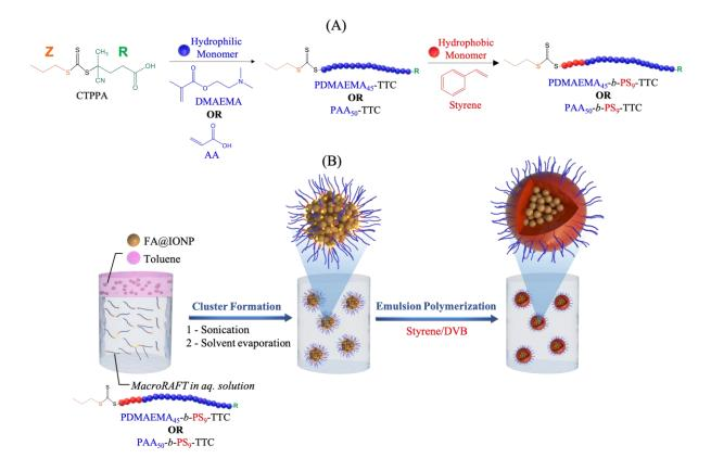
Scheme 1 – Schematic representation of (A) synthesis of amphiphilic block copolymers (PDMAEMA<sub>45</sub>-b-PS<sub>9</sub>-TTC or PAA<sub>50</sub>-b-PS<sub>9</sub>-TTC), and (B) IO cluster formation via emulsification/solvent evaporation and synthesis of magnetic latex particles via emulsion polymerization using the macroRAFT-stabilized clusters as seeds.
