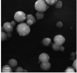
**Figure 7** – (A) TEM and (B) SEM micrographs of PAA@MLPs synthesized by seeded semi-batch emulsion polymerization of styrene with 23 wt% DVB (Exp 11, Table 2). Scale bar = 100 nm.
