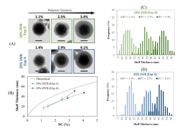
**Figure 5** – Evolution of the shell thickness with the polymer content for PDMAEMA@MLPs prepared by seeded emulsion polymerization of styrene in the presence of 10 or 20 wt% of DVB (Exp 3 and 4, respectively, Table 1). The theoretical shell thickness was calculated according to the equations 5 and 6.
