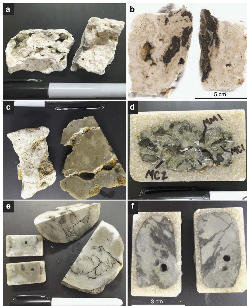
**Figure 2 | Photographs of cold seep carbonates.** (a,b) Hydrate Ridge samples exhibiting light and dark primarily carbonate phases. (c,d) Costa Rica cold seep carbonate with micrite (MM1) and clotted micrite (MC1,2) sample sites indicated. (e,f) Eel River Basin cold seep dolomite samples exhibiting similar light and dark colour variation as Hydrate Ridge samples. Permanent marker cap is 5-cm long.
