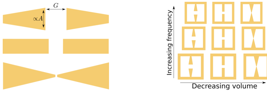
Figure 5: Left: based on the parallel-plate capacitor model, the capacitance is kept constant by keeping the same ratio A/G . Right: variation of the SRR shape with the two independent parameters (size and gap width).
