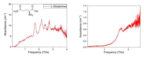
Figure 3: Spectrum of glutamine  $[C_5H_{10}N_2O_3]$  samples. Left - 6.8 µg of powder (volume of about 5 nL), right - 250 ng of dried solution (volume of dried solution of about 200 pL). We cut the spectrum at 2.5 THz for the dried solution because of the lower signal-to-noise ratio.
