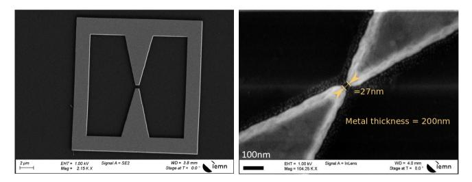
Figure 8: SEM image of a SRR (left) and close up view on a 27 nm gap (right).
