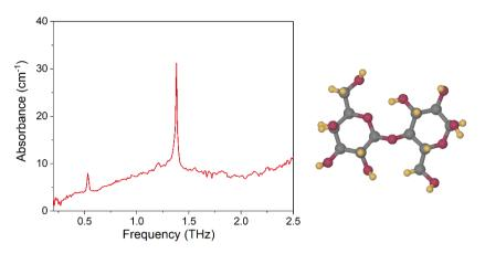
Figure 2: Left - spectrum of a powder of  $\alpha$ -Lactose monohydrate. The sample volume is ~ 15 nL corresponding to a mass of ~ 23  $\mu$ g. Right - schematic view of the lactose molecule.
