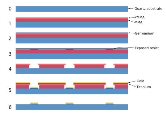
Figure 6: Step by step illustration of the fabrication process.
