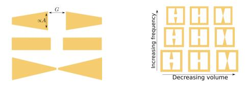
Figure 5: Left: based on the parallel-plate capacitor model, the capacitance is kept constant by keeping the same ratio A/G. Right: variation of the SRR shape with the two independent parameters (size and gap width).
