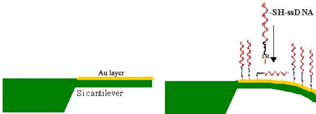
Fig.1 Principle of working of a nanomechanical biosensor
