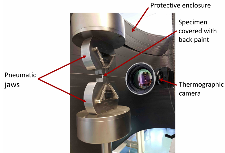
Figure 2: Experimental setup to measure the self-heating of the specimen during cyclic loadings.
