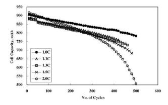
Figure 2. An example of accelerated capacity fading due to higher C-rates
