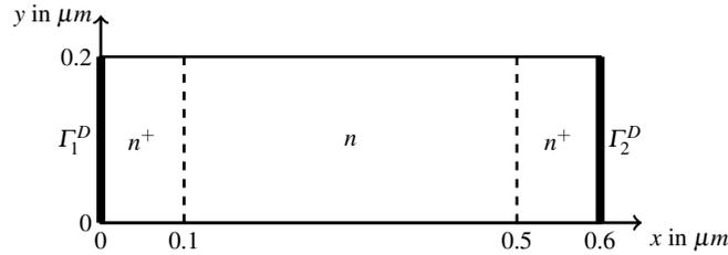
**Fig. 1** Geometry of the  $n^+nm^+$  ballistic diode.
