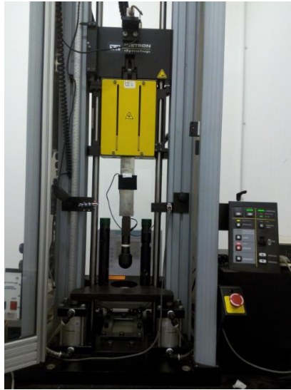
Fig. 5. Instrumented dropping weight impact tower.
