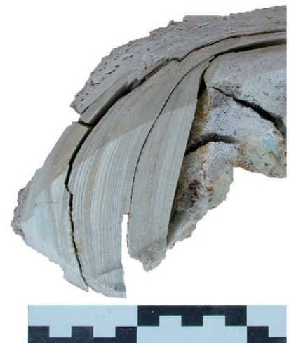
Figure 5: An alternate black/white laminated travertine (Facies A) from Roman baths, Jebel Oust, Tunisia.
