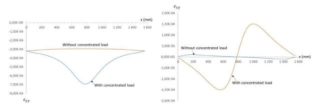
Fig. 30 PCW estimates at time t = 900 days for the evolutions of the local strain  $\varepsilon$ yy (left) and  $\varepsilon$ xy (right) versus abciss x in the middle height of a wall with viscous bricks: comparison between boundary conditions BC-1 and BC-2.
