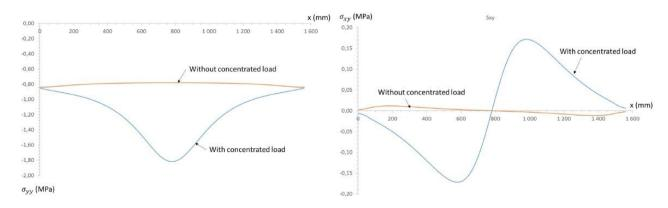
Fig. 26 PCW estimates at time t = 900 days for the evolutions of the local stress  $\sigma$ yy (left) and  $\sigma$ xy (right) versus abciss x in the middle height of a wall with viscous bricks: comparison between boundary conditions BC-1 and BC-2.
