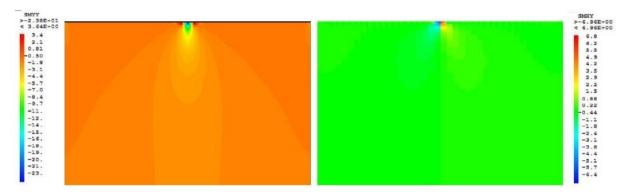
Fig. 24 Local normal (left) and shear (right) stress snapshots throughout a wall (with viscous bricks) under BC-2.
