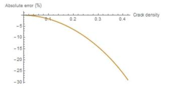
Fig. 9 Open cracks: percent errors between PCW and dilute estimates for the micro-cracked mortar's Young's modulus versus crack density either for t = 20 and 1000 days.
