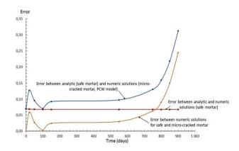
Fig. 22 Time evolutions of the error between analytic (safe mortar) and numerical (safe and microcracked mortar) solutions for vertical displacement uy at the top of the compressed wall
