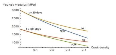
Fig. 8 Open cracks: PCW and dilute estimates for the microcracked mortar's Young's modulus versus crack density at instants t = 20 and 1000 days.
