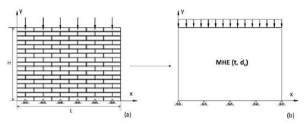
Fig. 19 Rigid bricks and viscoelastic mortar joints: Real (a) and equivalent homogenized (b) masonry panels subjected to a vertical distributed load applied at the top [56].
