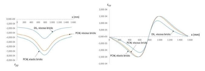
Fig. 31 Boundary condition BC-2: comparison between PCW and dilute estimates for the evolutions of normal and shear stresses versus x axis (wall with viscous bricks) and study of the effect of accounting for creep of bricks
