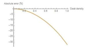
Fig. 5 Closed cracks: percent error between PCW and dilute estimates for the microcracked mortar's effective Young's modulus (t = 20 and 1000 days) versus crack density.
