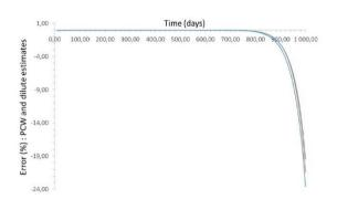
Fig. 17 Comparison between PCW and dilute estimates for effective properties of a masonry cell constituted by viscous bricks and microcracked mortars joints with open cracks which crack density evolves following a time power-law function.
