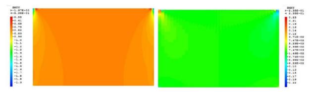
Fig. 25 Local normal (left) and shear (right) stress snapshots throughout a wall (with viscous bricks) under BC-1
