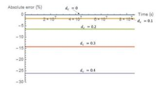
Fig. 10 Open cracks: percent errors between PCW and dilute estimates for the microcracked mortar's Young's modulus with different crack densities (dc = 0, 0.1, 0.2, 0.3 and 0.4) versus time.
