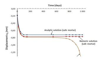
Fig. 21 Rigid bricks and viscoelastic mortar joints: Time evolutions of the local vertical displacement uy at the top of the panel.
