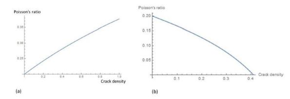
Fig. 2 Evolution of the PCW estimate for the effective "Poisson's ratio" of the microcracked mortar with crack density dc in the case of closed (a) and open (b) cracks.
