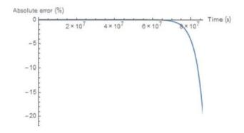
Fig. 13 Open cracks which crack density evolves following a time power-law function: percent error between PCW and dilute estimates
