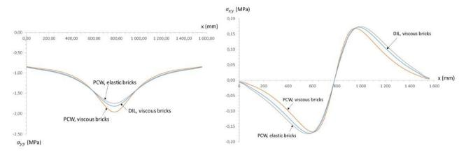
Fig. 27 Boundary condition BC-2: comparison between PCW and dilute estimates for the evolutions of normal and shear stresses versus x axis (wall with viscous bricks) and study of the effect of accounting for creep of bricks.
