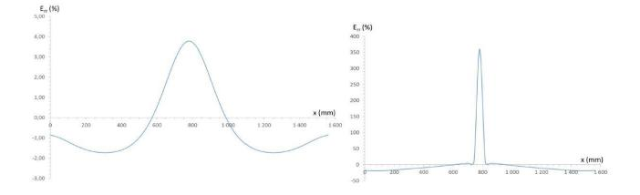
Fig. 29 Percent error between PCW estimates for local normal (left) and shear (right) stresses in the middle height of the wall: effect of bricks' creep.
