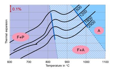
**Fig. 5.** Dilatometer courses for the given nominal heating rates in K s<sup>-1</sup> and indication of transformation areas (F – ferrite, P – perlite, A – austenite).
