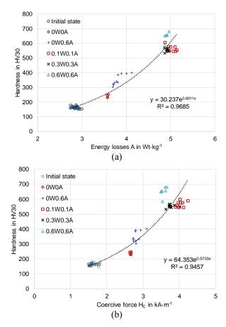
Fig. 16. Hardness of the given samples as a function of energy losses A (a) and coercive force  $H_C$  (b) with respective logarithmic equations.
