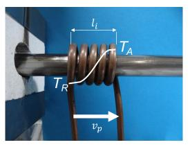
Fig. 3. Heating station with a given inductor coil and parameters determining the heating rate at a constant inductor power.
