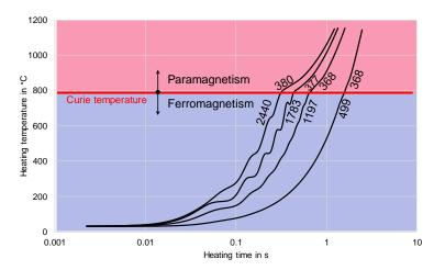
Fig. 4. Heating courses obtained during dilatometric experiments with the actual heating rates calculated below and above Curie temperature in K  $s^{-1}$ .
