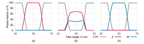
**Fig. 19.** Phase distribution along the tube length on the inner tube surface after the inductive heating (a), at the time point of 19.5 s during the cooling (b) and after the completed cooling (c).
