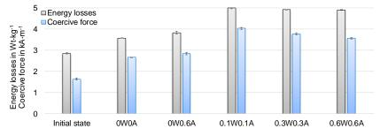
Fig. 15. Average values of the energy losses and coercive force for the given samples with standard deviation.
