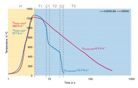
Fig. 9. Time-temperature-courses due to heat-treatments composed of inductive heating at 12 kW and spray cooling at the given cooling parameters in MPa with a feed rate of 16.7 mm s<sup>-1</sup>.
