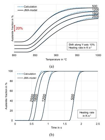
**Fig. 6.** Evolution of the austenite formation during the inductive heating with the given heating rates depending on (a) temperature – shift along the Y-axis of 10% - and (b) time from the start of the heating process according to calculated dilatometric data and to JMA-model.
