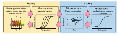
Fig. 17. Model allowing the inverse determination of the required parameters of heat-treatment based on target mechanical properties.
