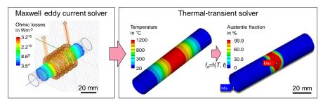
**Fig. 18.** Simulation of the inductive heating for a feed rate of  $16.7 \text{ mm s}^{-1}$  composed of the determination of ohmic losses due to inductive influence in Maxwell eddy current solver and generation of the temperature field along with calculation of the austenite fraction in the thermal-transient solver.
