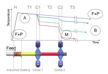
**Fig. 8.** Possible heat-treatment strategies to obtain different phase compositions under consideration of the parameters of the heat-treatment station (H – heating; T1, T2, T3 – air transportation stages; C1, C2 – water-air spray cooling circles).
