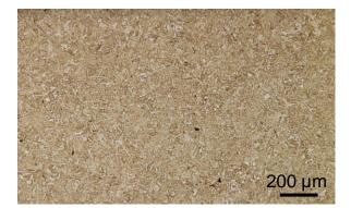
Fig. 7. Exemplary micrograph of the dilatometric sample exhibiting martensitic microstructure after heating with rate of 2500 K s<sup>-1</sup> and immediate quenching with a rate of 30 K s<sup>-1</sup>.
