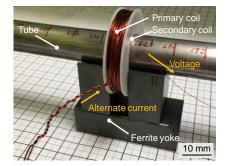
Fig. 13. Setup of the magnetic device composed for determination of the magnetic properties in the tube cross-sections.
