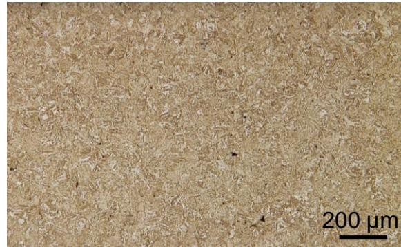
Fig. 7. Exemplary micrograph of the dilatometric sample exhibiting martensitic microstructure after heating with rate of 2500 \text{ K s}^{-1} and immediate quenching with a rate of 30 \text{ K s}^{-1} .
