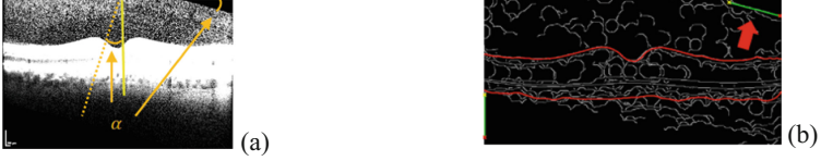
Fig. 4. Estimation of the incident light beam angle from the saturated image (a); linear segments (in green) extracted from the contour image through the Hough transform (b). (Color figure online)
