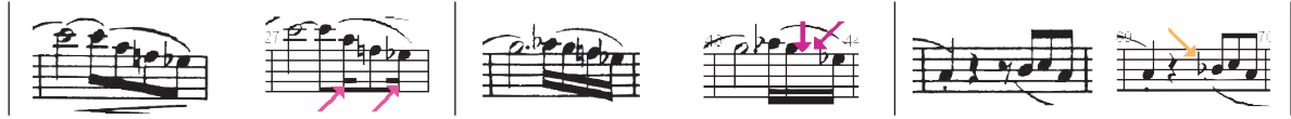
FIGURE 1: Examples of recognition errors provided by a commercial software [4]. On the left-hand side of each column, the original bar, on the right-hand side, the recognition results.
