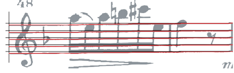
FIGURE 6: Accurate detection of warped staff lines.
