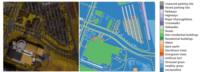
Fig. 3: Data from the DFC2018 dataset. Example of false RGB image (left) and the ground truth (right).
