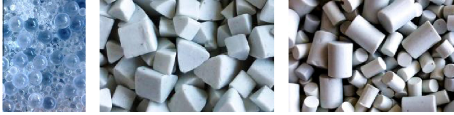
Fig. 2. Particles used to validate the void fraction measurement.
