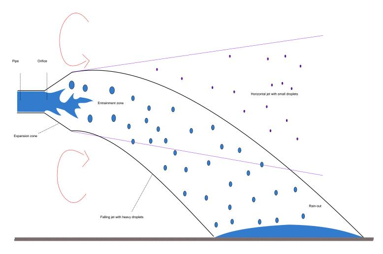
Figure 1: Schematic representation of flashing jet regions
