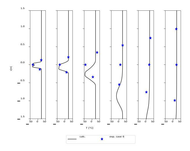
Figure 9: Comparison of several vertical profiles of temperature obtained by INERIS experiment (exp.) and the TEM numerical model (calc.) for case 6. The axial position of the profiles from left to right are: 0.5m; 1m; 2m; 3.5m; 5m; and 6.5m.
