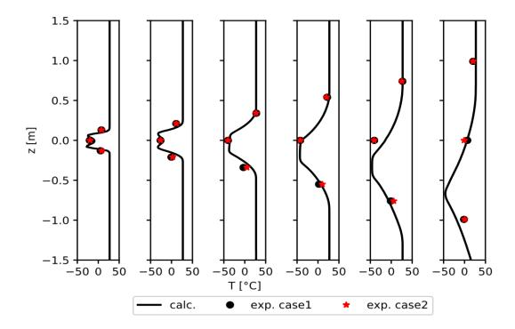
Figure 8: Comparison of several vertical profiles of temperature obtained by INERIS experiment (exp.) and the TEM numerical model (calc.) for case 1 & case 2. The axial position of the profiles from left to right are: 0.5m; 1m; 2m; 3.5m; 5m; and 6.5m.
