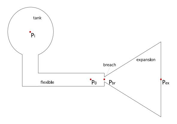
Figure 4: Schematic representation of flashing jet regions
