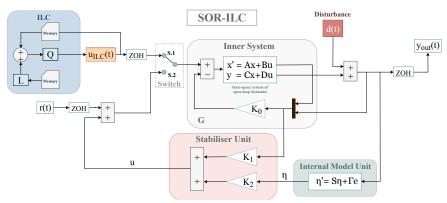
Fig. 1. SOR-ILC test model
