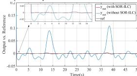
Fig. 7. System outputs with SOR-ILC (on/off)
