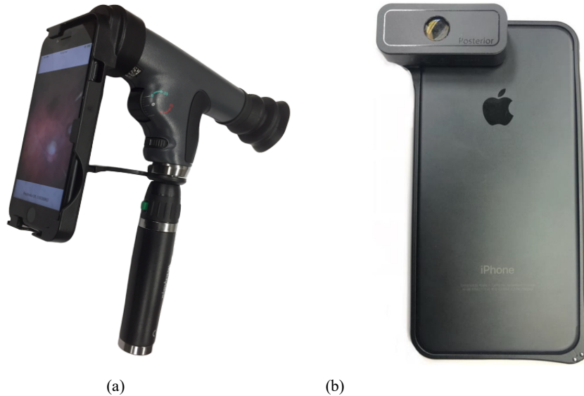
Figure 1. Pictures of commercially available lenses for smartphones: (a) WelechAllyn lens, and (b) D-EYE lens
