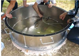
Installation of calibrated permeability interface and subwoofer
