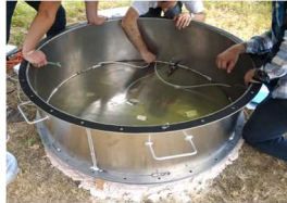
Installation of calibrated permeability interface and subwoofer
