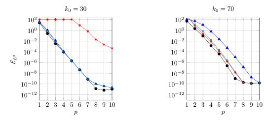
Figure 9:  $L^2$ -error (in %) for fixed frequencies as a function of the shape function order p for the classical (-\*-), alternative (-\*-) and Lorentz (-\*-) PMLs. Parameters: n=3, M=0.8 and  $\sigma_0=4\beta^2$ . Reference solution (-•-).
