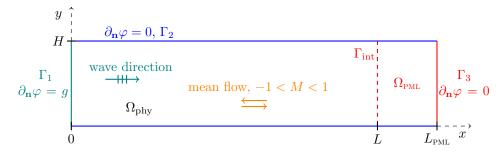
Figure 3: Sketch of the numerical case: 2D acoustic duct propagation in a uniform mean flow. The global domain is  $\Omega = \Omega_{phy} \cup \Omega_{PML}$  and the PML interface is  $\Gamma_{int} = \Omega_{phy} \cap \Omega_{PML}$ .
