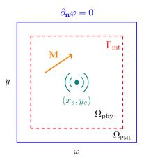
Figure 10: Sketch of the numerical case: 2D point source radiation in a cross flow with straight boundaries. The global domain is  $\Omega = \Omega_{\rm phy} \cup \Omega_{\rm PML}$  and is delimited by respectively L and  $L_{\rm PML}$ .
