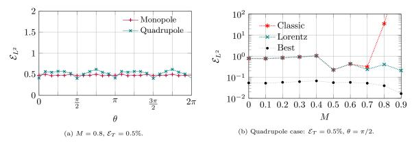
Figure 18:  $L^2$ -error (in %) for the circular PML as a function of the flow angle and Mach number.
