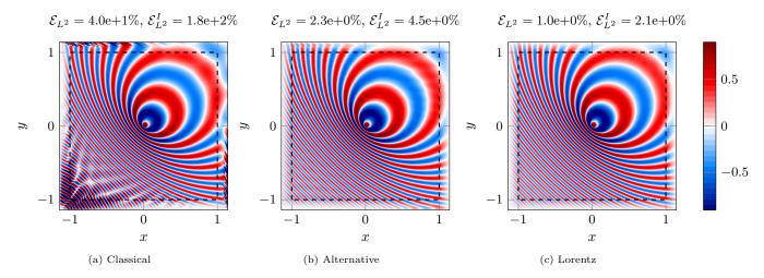
Figure 11: Real part of the numerical solution at  $\omega = 6\pi$ , M = 0.8 and  $\theta = \pi/4$  for the three PML models with  $\sigma_0 = \beta$ .
