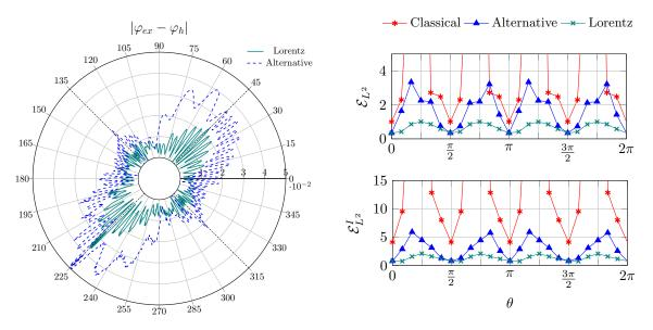
Figure 12: Polar diagram of the local error along the PML interface Figure 13: Domain and interface  $L^2$ -errors (in %) as a associated to Figures 11b and 11c. function of the flow angle  $\theta$  for M=0.8 with  $\sigma_0=\beta$ .
