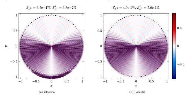
Figure 17: Real part of the numerical solution at  $\omega = 20\pi$ , M = 0.8 and  $\theta = \pi/2$  for the unstable and stable PML models with  $\sigma_0 = \beta$ .
