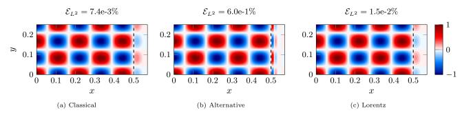
Figure 7: Propagative mode:  $k_0 = 70$ . Real part of the numerical solution for the three formulations. Reference  $L^2$ -error:  $1.3 \times 10^{-3} \%$ . Mach number M = 0.8, input mode n = 3, shape function order p = 4. The dashed line (---) is the PML interface.
