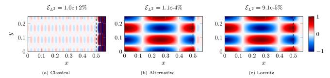
Figure 6: Inverse upstream mode:  $k_0 = 30$ . Real part of the numerical solution for the three formulations. Reference  $L^2$ -error:  $9.1 \times 10^{-5} \%$ . Mach number M = 0.8, input mode n = 3, shape function order p = 4. The dashed line (- - - ) is the PML interface.
