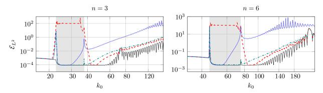
Figure 8:  $L^2$ -error (in %) for the classical (---), alternative (-----) and Lorentz (-----) PMLs. Parameters: M=0.8, p=4 and  $\sigma_0=4\beta^2$ . The shaded areas highlight inverse upstream propagation. Reference solution (-----).
