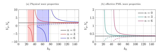
Figure 4: Adimensional phase  $V_p$  (plain lines) and group  $V_g$  (dashed lines) velocities for three propagative modes  $n = \{0, 3, 6\}$  and M = 0.8. The shaded areas highlight the inverse upstream regime.
