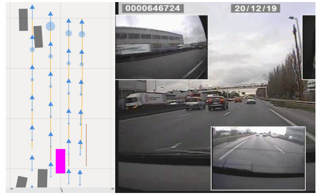
Fig. 6: On the left, tracking results (blue) and measurements (orange for FrontCam, brown for AVM) are displayed in a bird-eye view. On the right, the context cameras.
