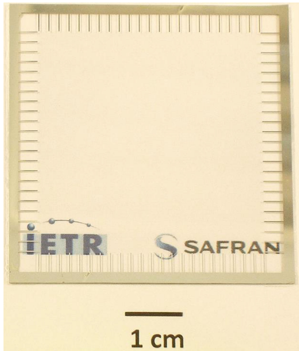
Fig. 7. Picture of the micrometric mesh silver/titanium film with 92 peripheral connected silver/titanium ribbons printed onto a 50.8 \text{ mm} \times 50.8 \text{ mm} \times 0.7 \text{ mm} soda-lime glass substrate. Sample is placed above the companies logos.
