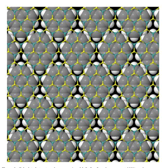
Figure 3. Calculated structure for pyrene in a  $MoS_2$ -3 × 3 surface array at 100% surface coverage, the most stable packing configuration. Pyrene atoms are shown with atomic van der Waals radii, showing the complete surface protective layer. Experimentally we calculate pyrene is forming between two and three layers.
