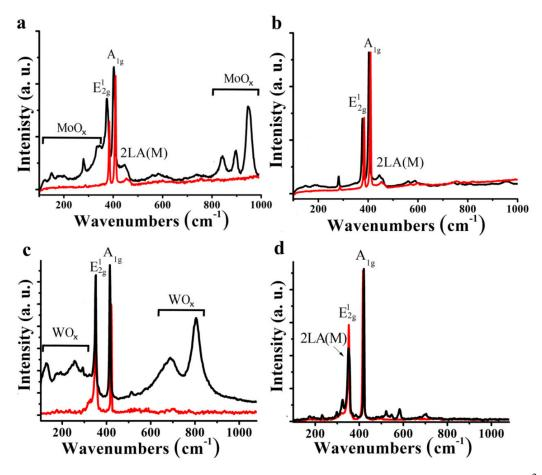
**Figure 4.** Raman spectra acquired at ambient conditions upon excitation at 514 nm with 0.1 mW/4  $\mu$ m<sup>2</sup> (red line) and 0.9 mW/4  $\mu$ m<sup>2</sup> (black line) laser radiance for (**a**) exfoliated MoS<sub>2</sub>, (**b**) MoS<sub>2</sub>/pyrene 1a, (**c**) exfoliated WS<sub>2</sub>, and (**d**) WS<sub>2</sub>/pyrene 1b. The E<sup>1</sup><sub>2g</sub>, A<sub>1g</sub>, and 2LA(M) peaks in the black spectra are downshifted due to laser heating.
