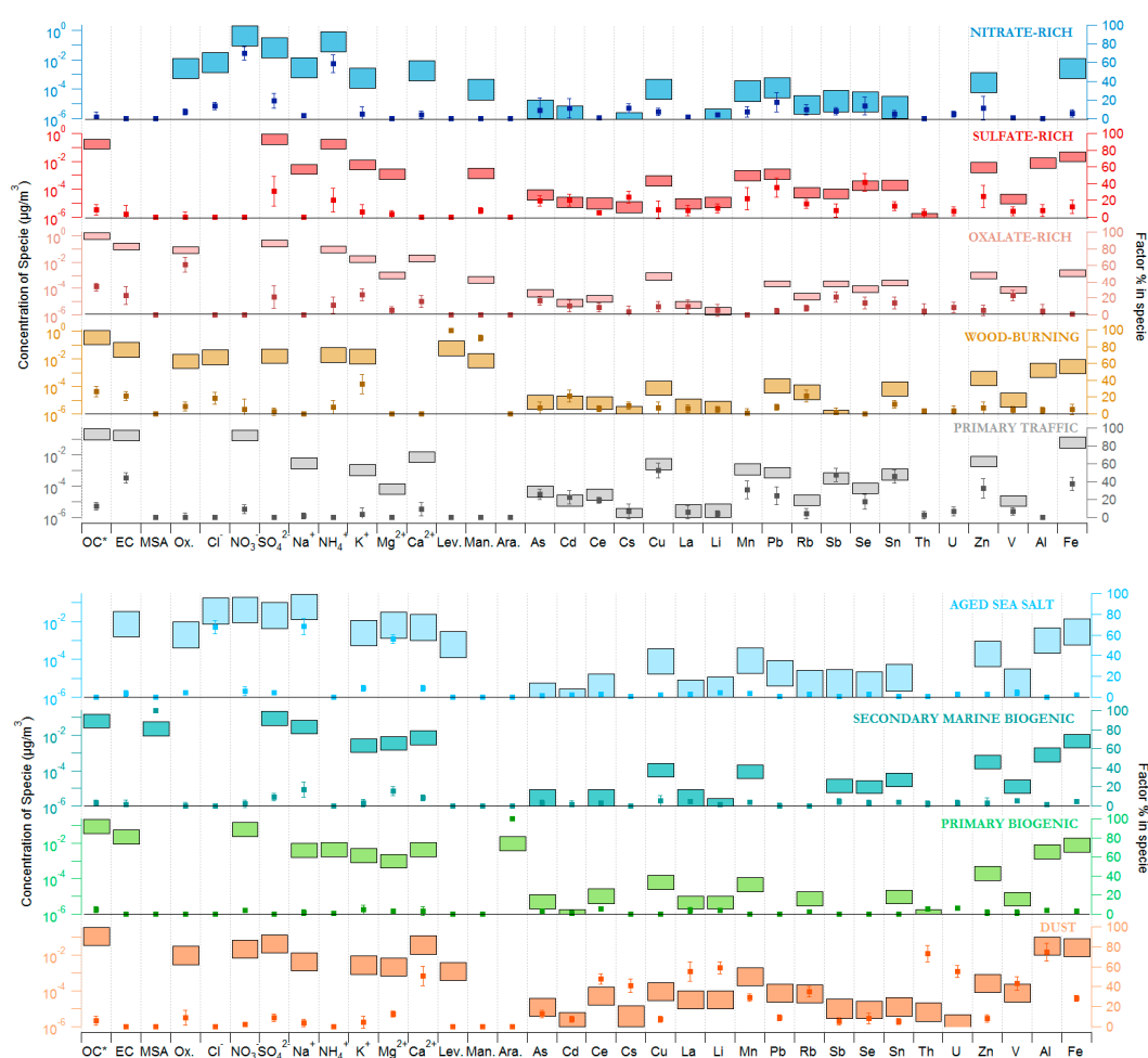
Figure 1. Chemical profiles of the PMF (Positive Matrix Factorization) factors obtained from the constrained bootstrap analysis. Bars (left axis) correspond to the InterQuartile Range (defined as p_{25} and p_{75} ) of concentration values in the profile; markers with error sticks correspond to the median ( \pm IQR) of factor percentage in each specie.
