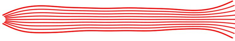
(a) Mode 12 with 1D model ( $f = 1621 \text{ Hz}$ )
