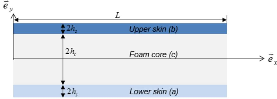
Figure 1: Two-dimensional representation of the sandwich column
