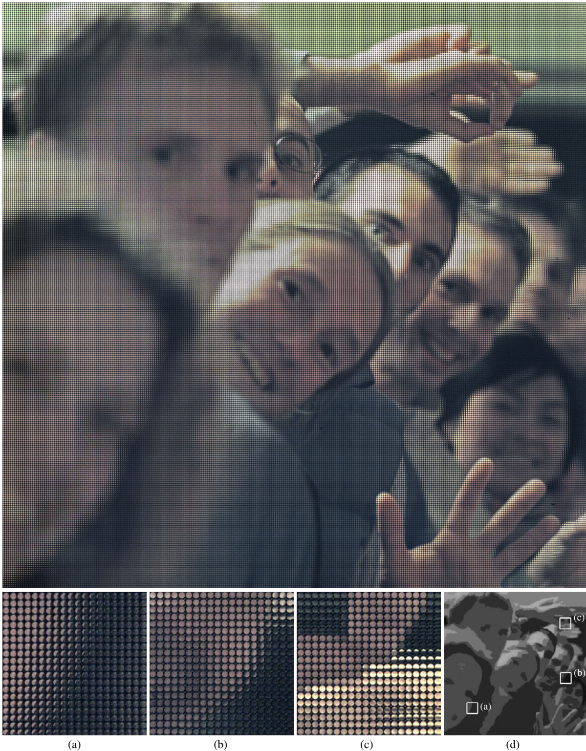
Figure 13: A complete light field captured by our prototype. Careful examination (zoom in on electronic version, or use magnifying glass in print) reveals 292 \times 292 microlens images, each approximately 0.5 mm wide in print. Note the corner-to-corner clarity and detail of microlens images across the light field, which illustrates the quality of our microlens focusing. (a), (b) and (c) show magnified views of regions outlined on the key in (d). These close-ups are representative of three types of edges that can be found throughout the image. (a) illustrates microlenses at depths closer than the focal plane. In these right-side up microlens images, the woman's cheek appears on the left, as it appears in the macroscopic image. In contrast, (b) illustrates microlenses at depths further than the focal plane. In these inverted microlens images, the man's cheek appears on the right , opposite the macroscopic world. This effect is due to inversion of the microlens' rays as they pass through the world focal plane before arriving at the main lens. Finally, (c) illustrates microlenses on edges at the focal plane (the fingers that are clasped together). The microlenses at this depth are constant in color because all the rays arriving at the microlens originate from the same point on the fingers, which reflect light diffusely.
