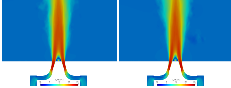
Fig. 7 Mean axial velocity fields for cases A-NR (left) and B-NR (right) in the central vertical plane.
