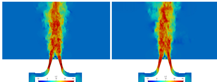
Fig. 6 Instantaneous axial velocity fields for cases A-NR (left) and B-NR (right) in the central vertical plane.
