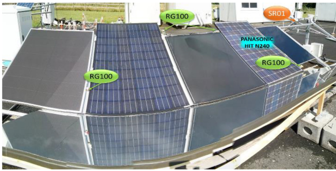
Fig. 4. Characterization test bench equipped with sensors and flat reflectors, SIRTA observatory.
